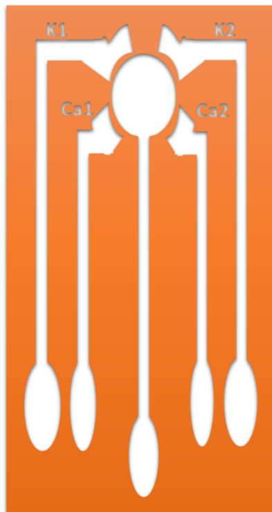
Figure 1. Scheme of the nano sensor with four sensing areas: K1, K2, Ca1, Ca2.
