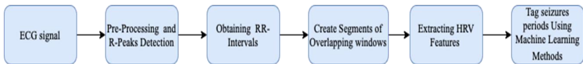
Figure 1. flow diagram of the proposed methodology. First, the ECG was inspected by identifying the R-peaks with 4 different detectors over 30 records and their performances were measured. Afterwards, the intervals between subsequent R-peaks were obtained yielding the RR intervals. The last step consisted of computing the HRV features and evaluate our ability to detect seizures' periods trough deep machine methods.
