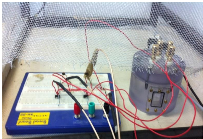
Figure 2: Our experiment system includes voltage clamp and pressure chamber, connected via electrodes. Current, voltage and pressure signals are acquired, displayed and processed using MATLAB.
